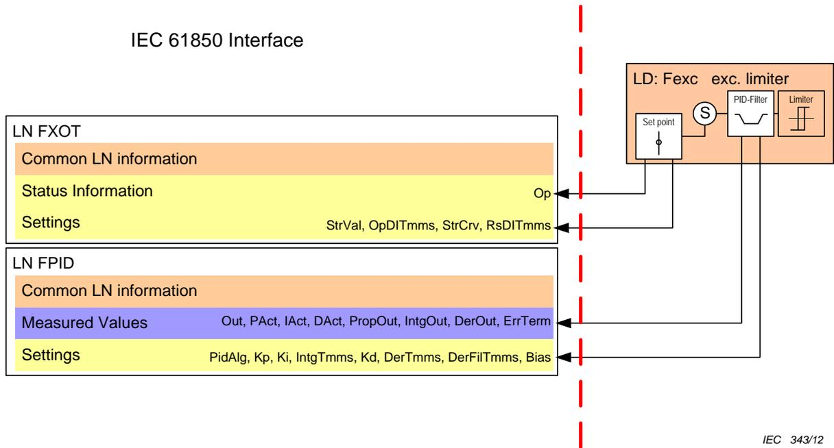
Figure 10 – Superimposed regulators, over-excitation limiter
