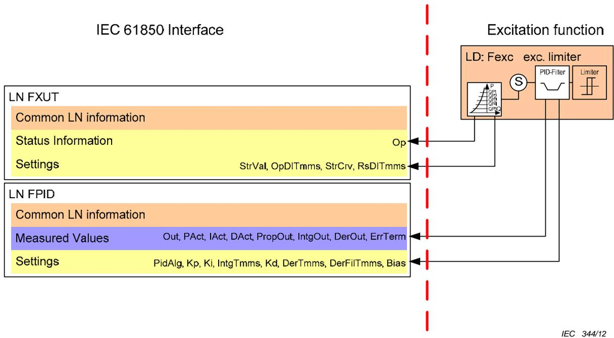
Figure 11 – Superimposed regulators, under-excitation limiter
