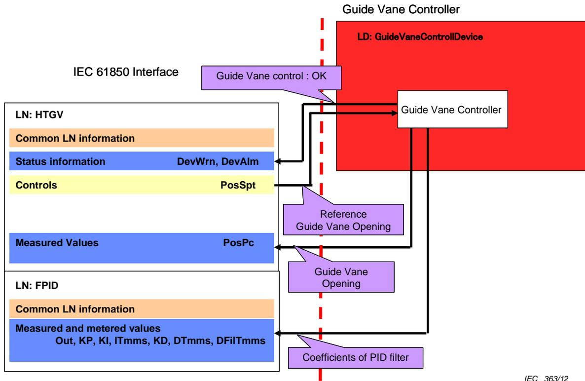
Figure 30 – Guide vane controller
