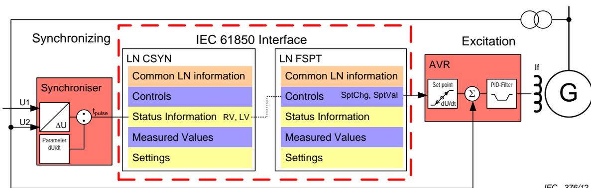
Figure 43 – Example of mapping of the pulse time in IEC 61850
