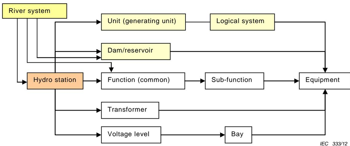
**Figure 1 – Structure of a hydropower plant**
