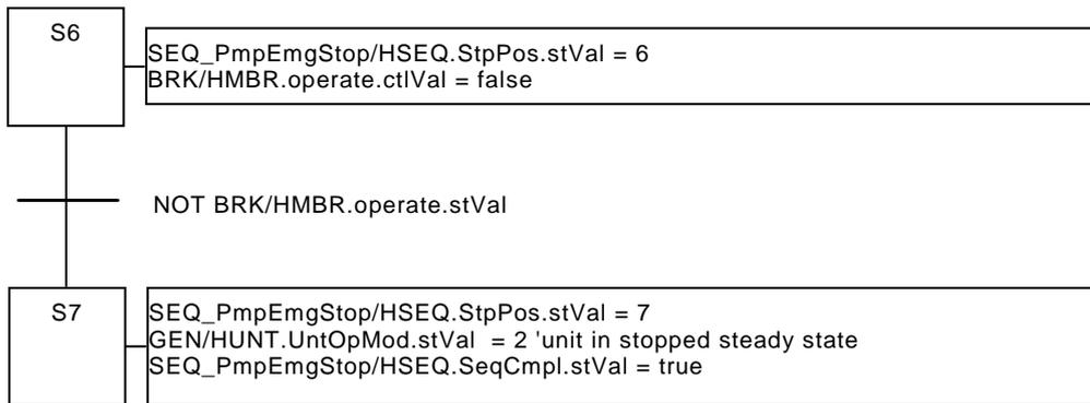
**5.4.7 Shutdown sequence from a state "Synchronous Condenser (SC) mode in pump direction" to a state "stopped"**
