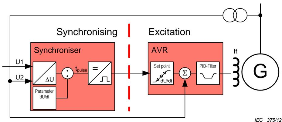
Figure 42 – Example of traditional voltage adjusting pulses
