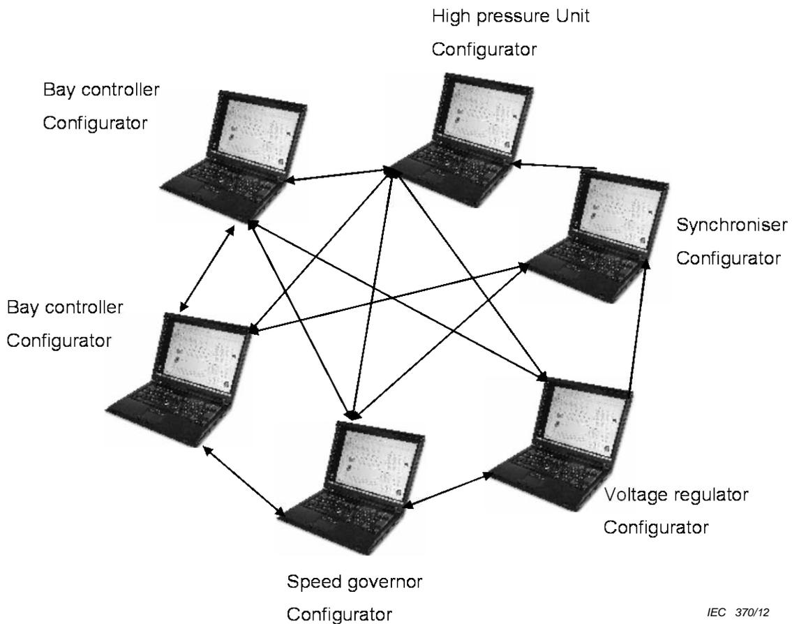
**Figure 37 – Exchange of ICD files between system configurators**
