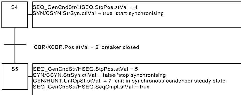
**5.4.3 Start sequence from a state "Synchronous Condenser (SC) mode in Pump direction" to a state "Pumping"**
