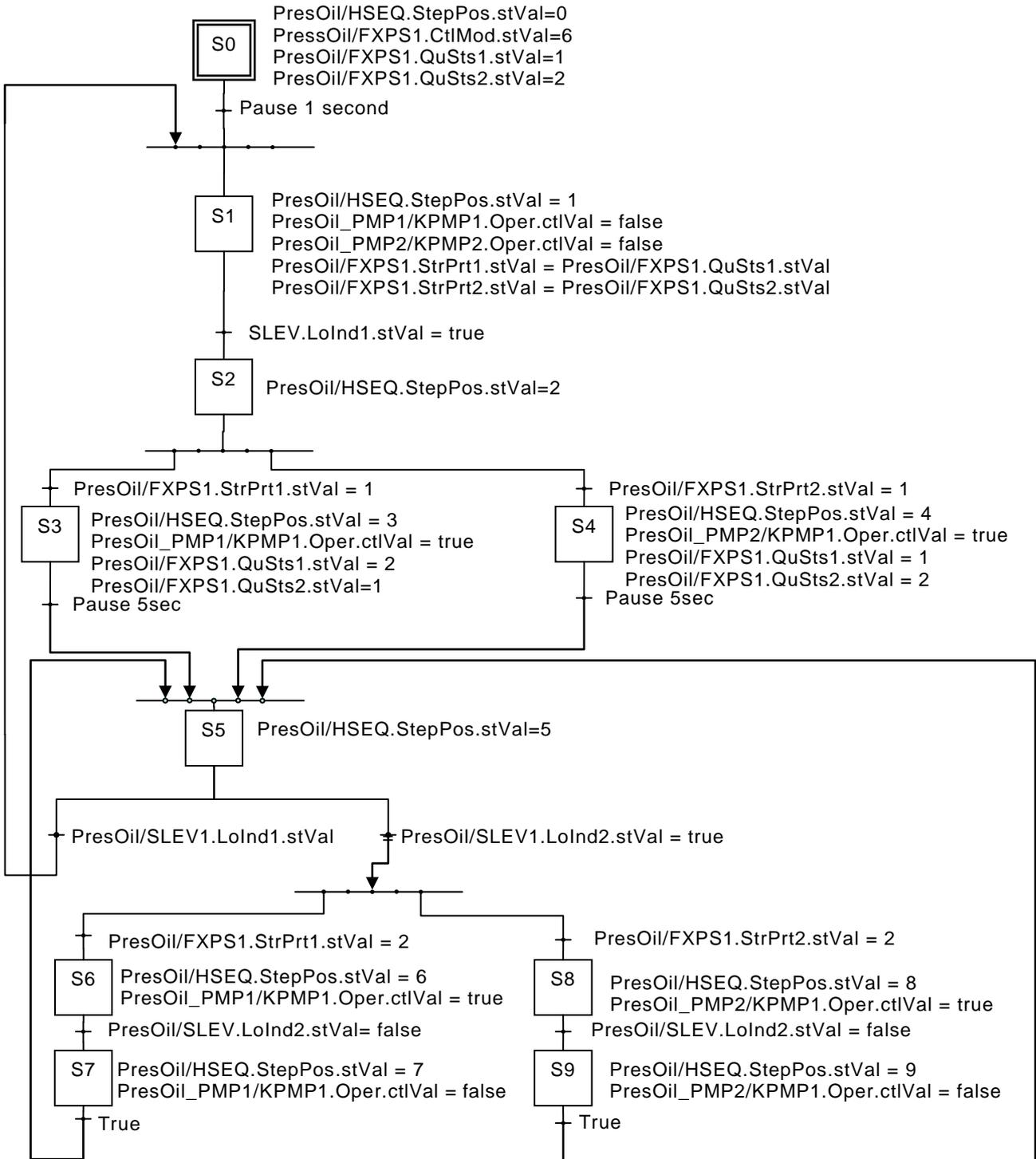
Figure 35 – Example of pump priority start logic sequence
