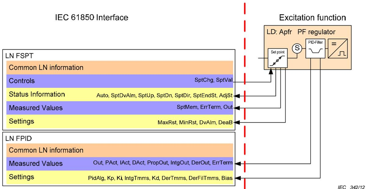
Figure 9 – Superimposed regulators, power factor regulator
