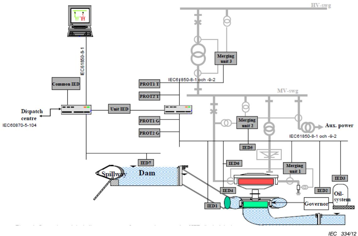
Figure 2 – Simplified network of a hydropower plant
