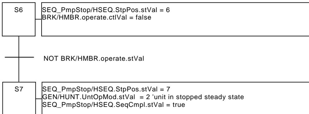
**5.4.6 Emergency shutdown sequence from a state "pumping" to a state "stopped"**
