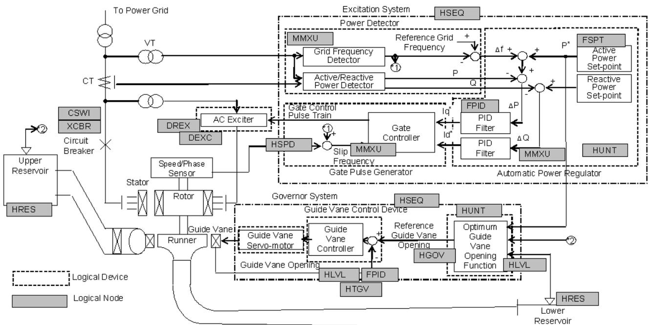
Figure 23 – Typical block diagram in pumping operation
