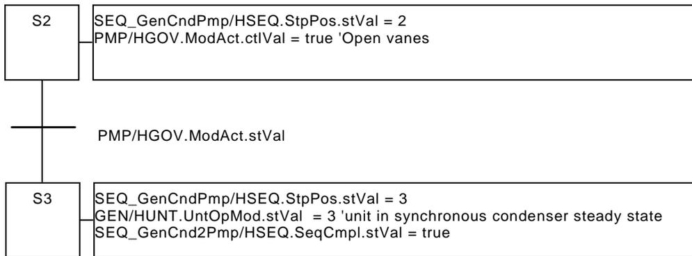
**5.4.4 Mode Transition sequence from a state "Pumping" to a state "Synchronous Condenser (SC) mode in Pump direction"**
